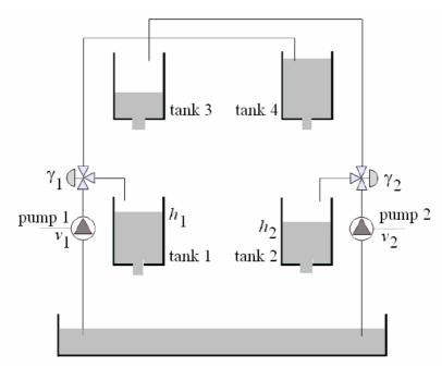
Figure 1. Schematic diagram of quadruple-tank process.
