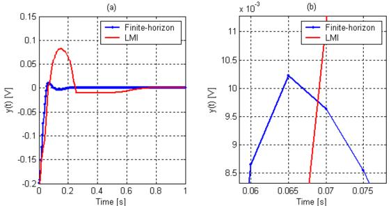
Figure 5. (a) Comparison of the presented solutions:  $K_{real} = 0.90 K_{nominal}$  without robust treatment. (b) Constraint violation detail.
