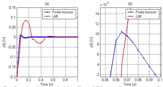
Figure 7. (a) Comparison of the presented solutions:  $K_{real} = 0.85K_{nominal}$  without robust treatment. (b) Constraint violation detail.
