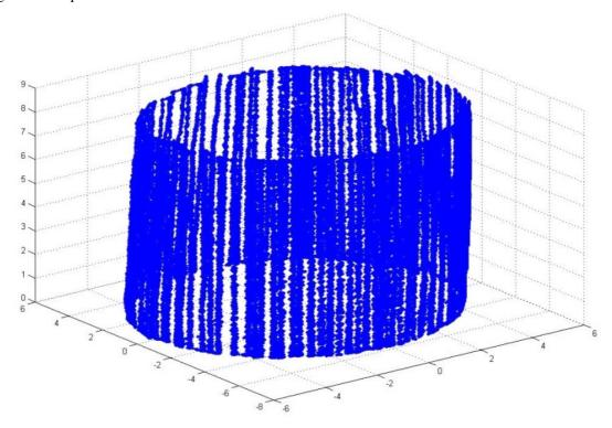
Figure 7. Acquired points representing a cylindrical surface.
