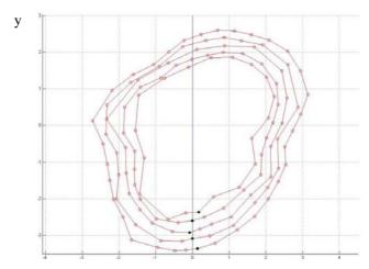
Figure 4. Selecting process for numbering the CM in order to draw the NURBS curve.
