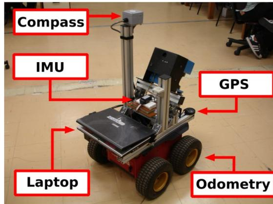
Figure 3. Equipments used in the real experiments.
