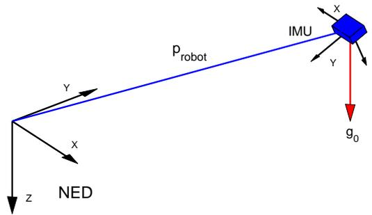
Figure 1. Gravity vector projection over the IMU axes.
