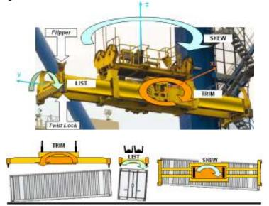
Figure 2. Spreader movements
