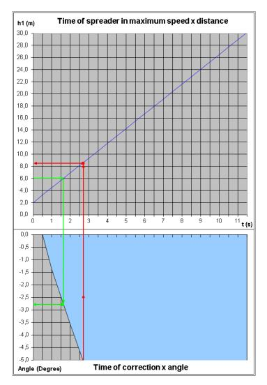
Figure 9. Correlation of the travel of the spreader and the angle corrected in the LIST movement
