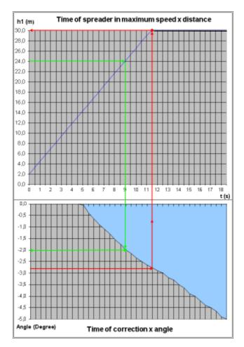
Figure 10. Correlation of the travel of the spreader and the angle corrected in the TRIM movement
