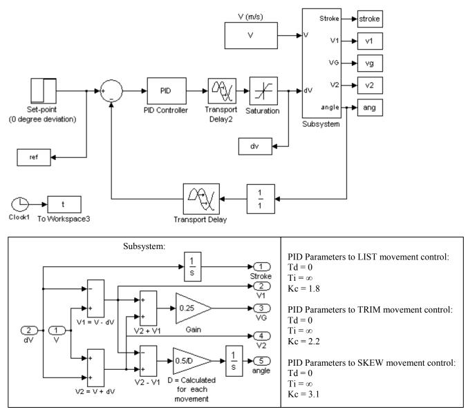
Figure 8. Closed loop control to TRIM, LIST e SKEW movements
