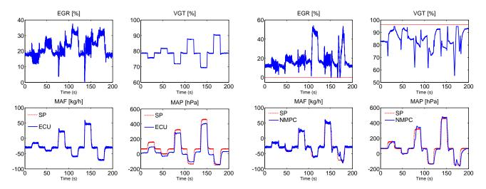
Figure 6. ECU's response (left) and the parameterized NMPC scheme (rigth) for a step sequence.
