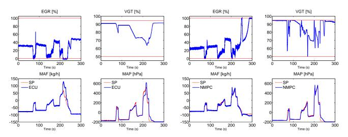
Figure 7. Experimental results showing the ECU's response (left) and the parameterized NMPC scheme (rigth) under the extra-urban part of the NEDC.
