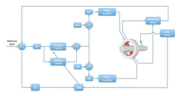
Figure 5. Feedforward associated with feedback control strategy for the magnetic actuator system.
