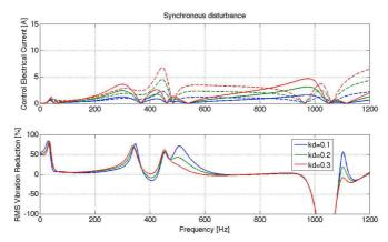
Figure 10. Control current (A) and RMS vibration reduction (%) behaviour in a range of synchronous frequency for AMB#1 (dashed line) and AMB#2 (solid line).
