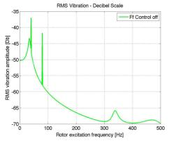
Figure 6. Frequency response of the rotor model with the subsynchronous (40 Hz) and synchronous (80 Hz) disturbances and with the feedforward control off (Ff Control off).
