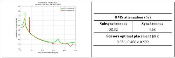
Figure 8. Frequency response and results for the rotor model with three error sensors placed in the optimal positions along the shaft.
