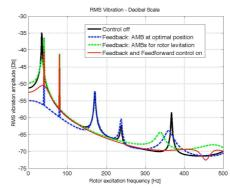
Figure 11. Frequency response comparisson to the different control systems applied to similar rotor models.
