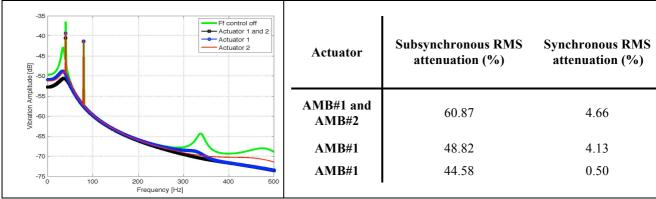
Figure 7. AMB selection from the rotor theoretical model.
