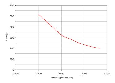
Figure 9. Time for the solution powder-processing operation fulfilled in the tank2 in function of heat supply rate.
