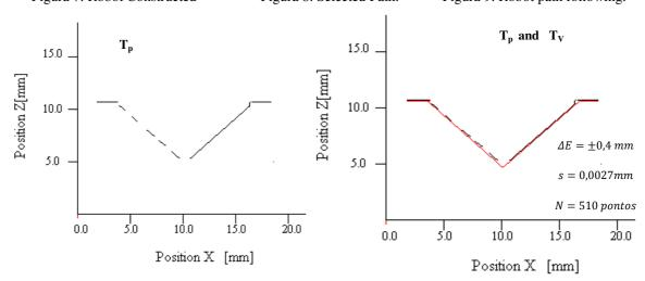
Figure 10. Path followed by the robot in the X-Z plane(Tp)
