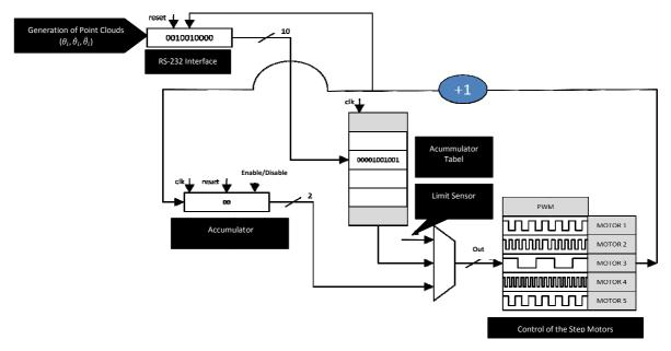
Figure 5. Block Diagram of the Robot Controller System.
