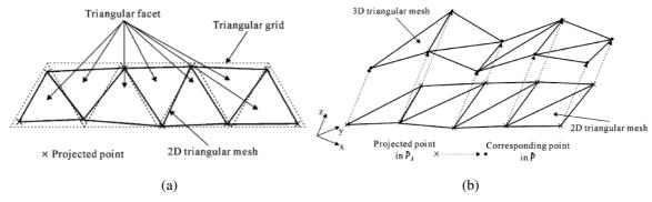
Figure 4. (a) 2-D triangular mesh constructed from the projected points next to nodal points repositioning. (b) 3-D triangular mesh is constructed based on its corresponding 2-D triangular mesh.
