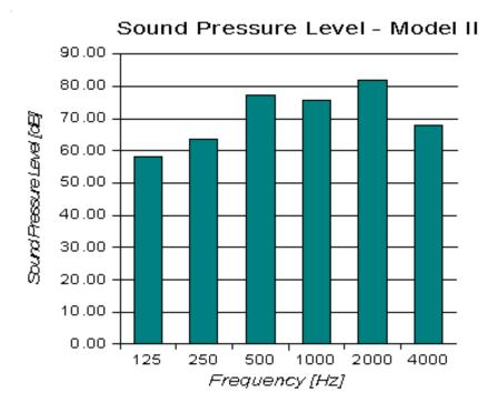
Figure 6. Average sound pressure level to the halls of the Model II
